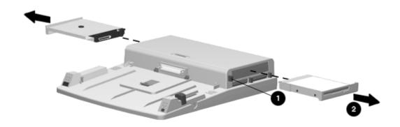
Figure 6-5. Removing a Mass Storage Device
